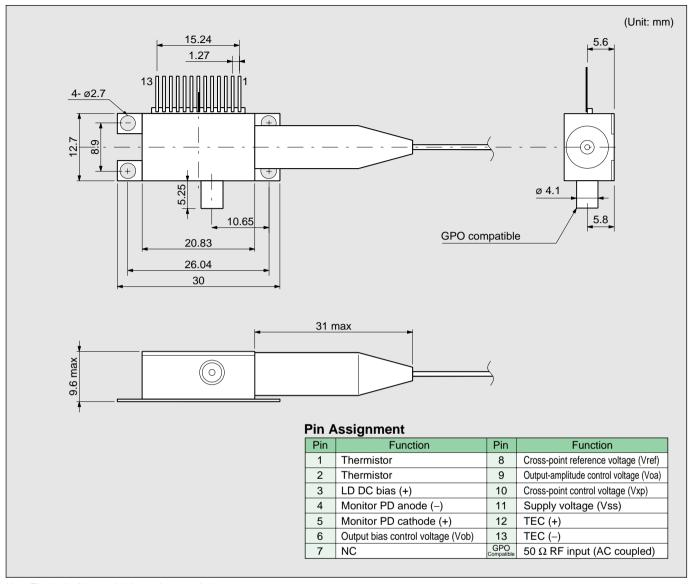
Note: The body of the module has to be grounded.
